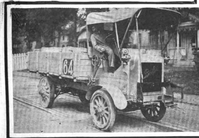
The Berliet entry was equipped with rubber tires on the front and steel tires on the rear wheels
